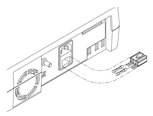
Figure 4: Fuse Removal
