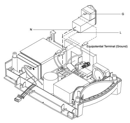
Figure 8: Power Entry Module
