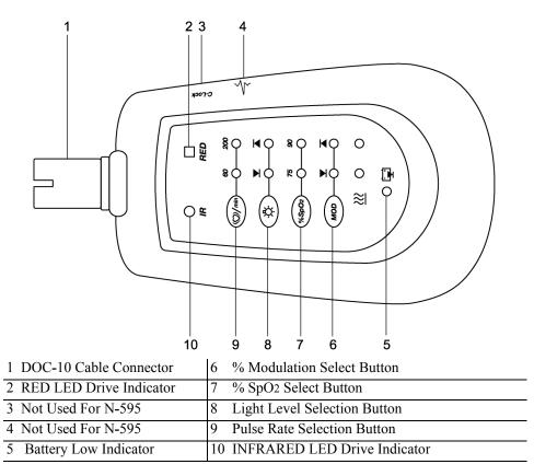
Figure 3: SRC-MAX OxIMAX Oximetry Tester
