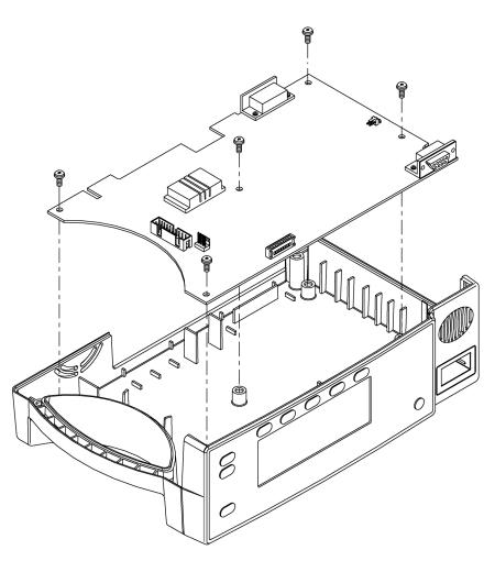
Figure 12: User Interface PCB
