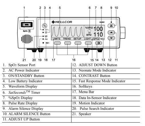
Figure 1: N-595 Front Panel
