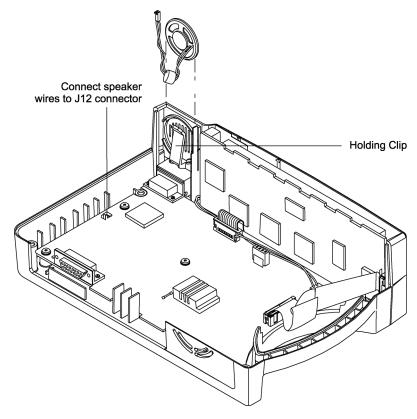
3. Pull the holding clip back from the speaker and lift the speaker out of the top case.
