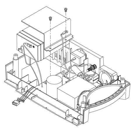
Figure 7: Removing the Battery
