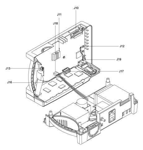
Figure 6: Separating Case Halves
